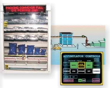
The "Midi" is one of our four "standard footprint" ROE-LIFT® Accumulators. Its time tested and patented design provide a reliable, high speed and high volume accumulation solution. By standardizing the length and width and building to your height and accumulation requirements, we are able to offer the Midi at a substantial cost savings over other accumulation methods.
